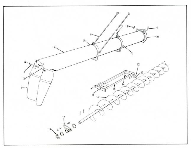
BIN UNLOADING CONVEYOR Used on Serial No. B-30601 & up
