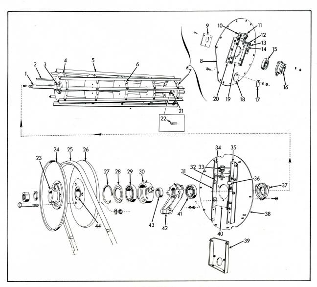
CYLINDER Used on Serial No. 69101 & up
