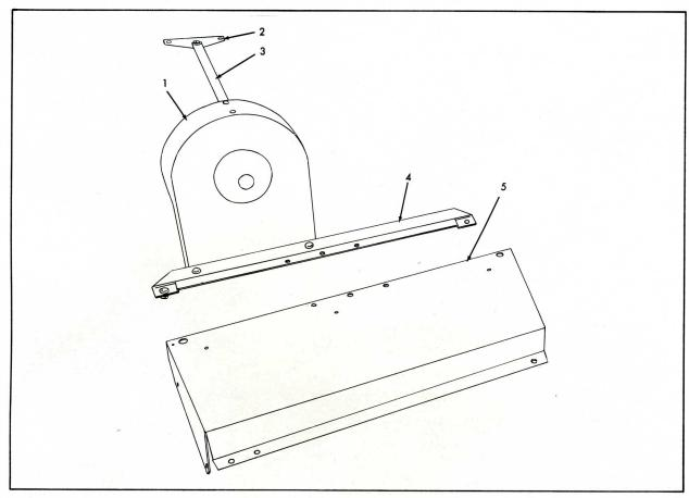
UNLOADING CONVEYOR BELT SHIELD Used prior to Serial No. B-30601
