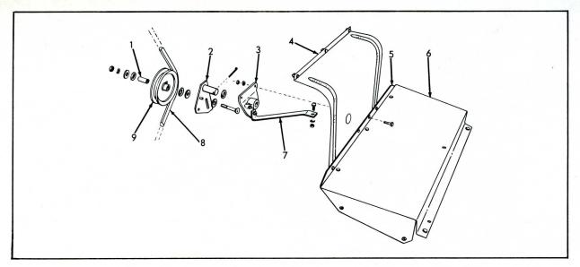
CONVEYOR BELT IDLER & SHIELD Used on Serial No. B-30601 & up
