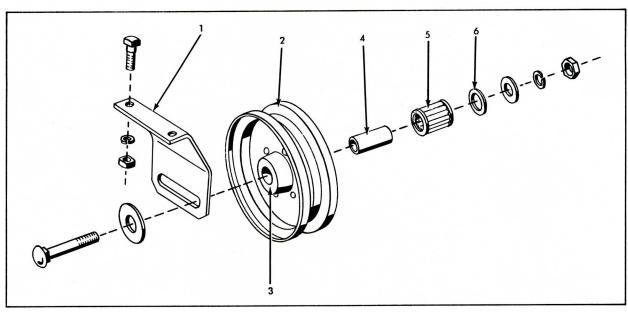
BIN CONVEYOR IDLER Used prior to Serial No. B-30601
