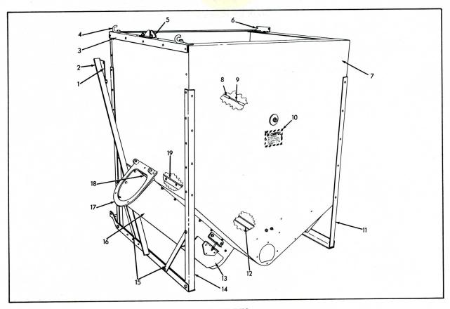
GRAIN BIN L.H. Front View Used on Serial No. B-30601 & up
