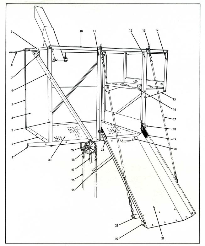
BAGGING ATTACHMENT R.H. Rear View Used prior to Serial No. B-30601
